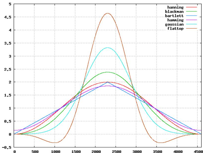
Figure 17.1: Spec and FFT window functions (Gaussian order = 4)
