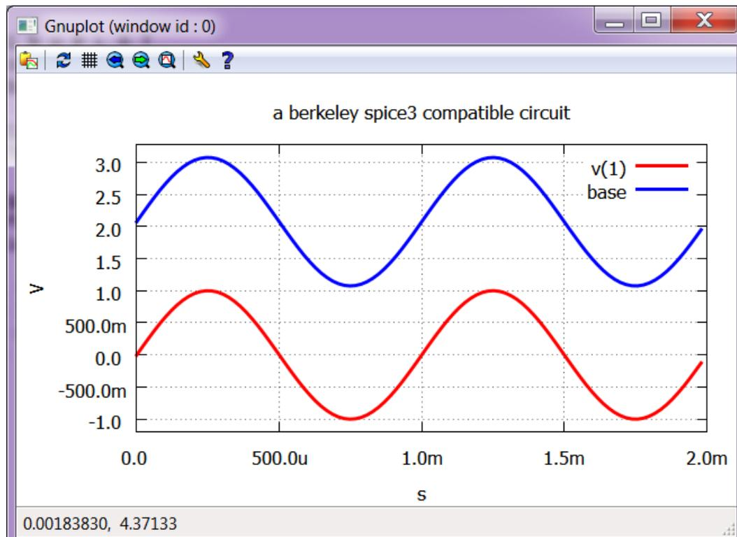
Figure 21.2: node 1 and node 'base' versus time
