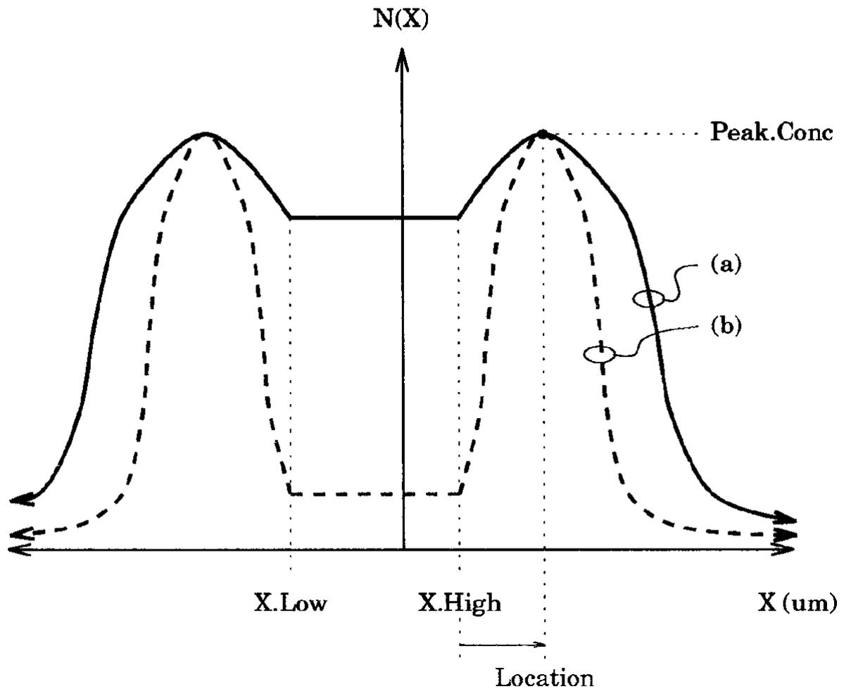
Figure 30.1: 1D doping profiles with location  $> 0$ .
