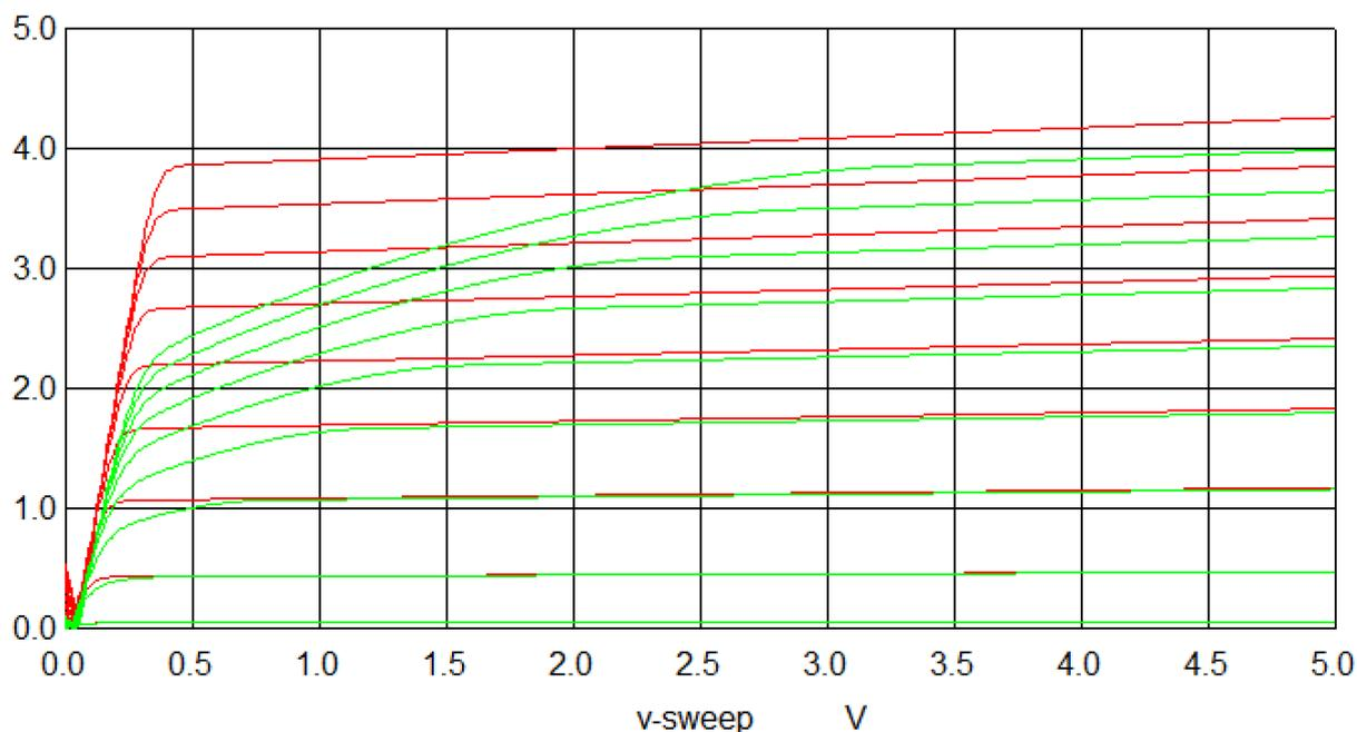
Figure 8.1: Output characteristic with and w/o Quasi-Saturation
