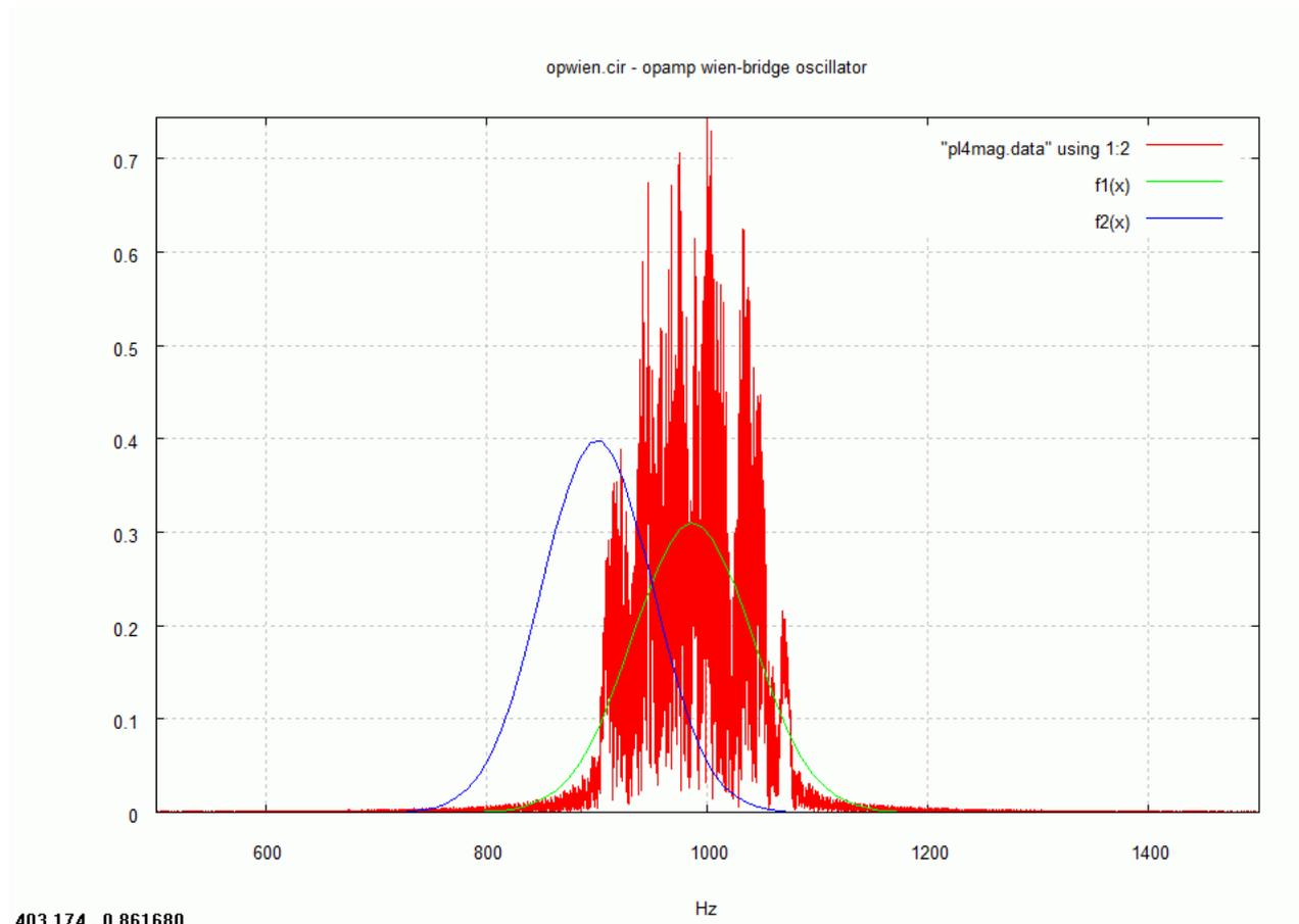
pl4mag.data is the simulation data,  $f2(x)$  the starting curve,  $f1(x)$  the fitted Gaussian distribution.
